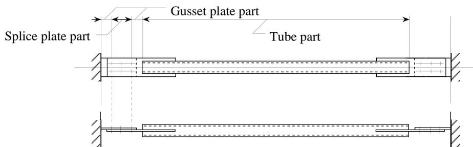
Fig. 1 Axially compressed tube with single shear through-gusset connection
